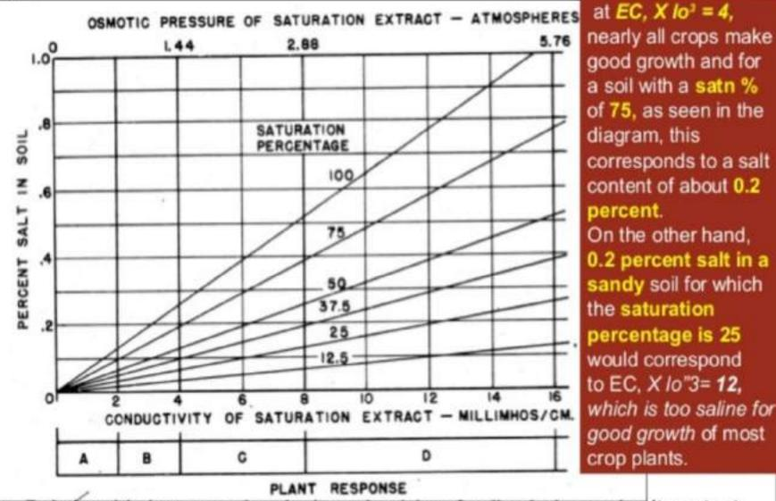
at EC,  $X lo^{3} = 4$ , nearly all crops make good growth and for a soil with a satn % of 75, as seen in the diagram, this corresponds to a salt content of about 0.2 percent. On the other hand, 0.2 percent salt in a sandy soil for which the saturation percentage is 25 would correspond
